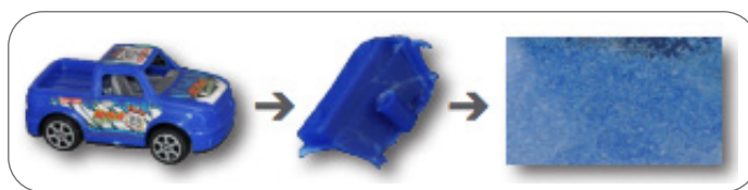
Figure 1. Original toy, subdivision and final ground powder.
