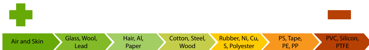
Figure 6. Triboelectric charge potential of common materials and particles in the laboratory
